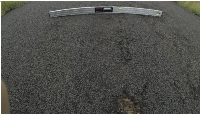
Avoid distortions created by fish eye or wide angle lens cameras mounted on car exterior. Use of level above is ineffective
